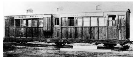
One of the two Gloucester Brake/2 nd /3 rd Composites based on Cleminson's principle - WHR 186 (Arch 0186)
