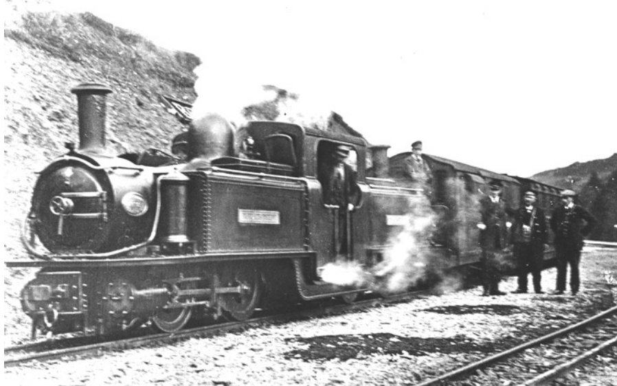
James Spooner at Beddgelert at about the time the complete railway opened. The Curly-roofed bogie brake next to the loco was what then was the only one of the three such vehicles surviving in its original form, F.R. Van No. 3. F.R. Bogie carriages are visible beyond; unfortunately 'staff' were standing in the wrong place, preventing identification! John Keylock collection. WHR 104
